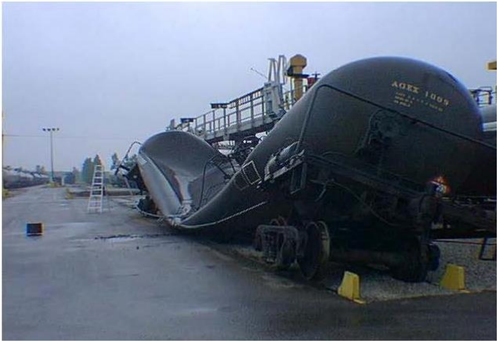
TANK CAR IMPLOSION CAUSED BY CONDENSING STEAM
